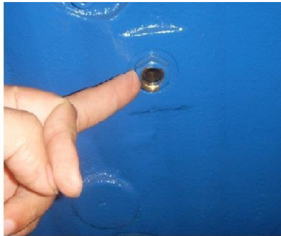
the window on the gearbox
