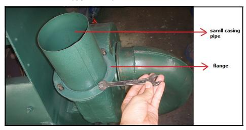
2. At last cover the big bend pipe on the small casing pipe.
