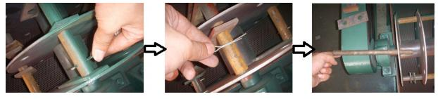
Install the new hammer sheets according to the original order.
