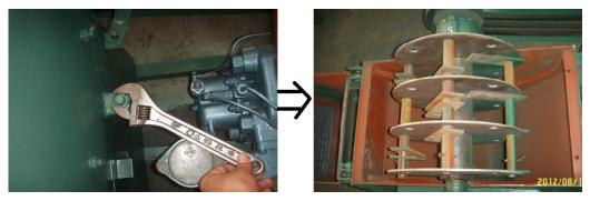
Remove the sieve, the replace a new one.
