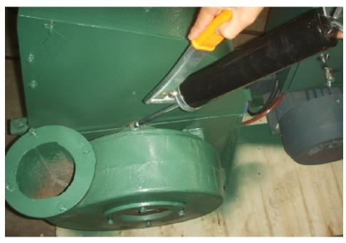
2. Lubricate the pulley and fan.
