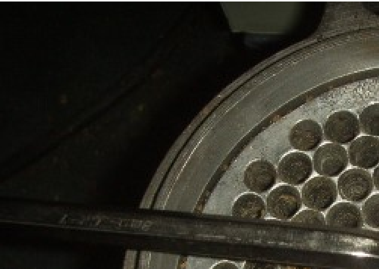
05 – Loosen the not in the center of the die
